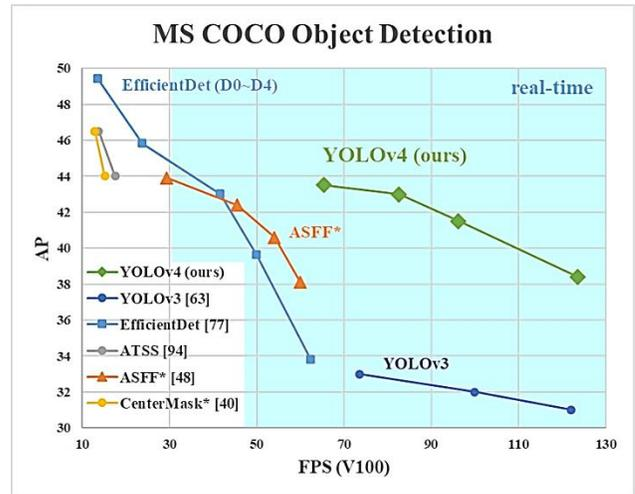
Figure 5. Comparison of different architectures with YOLOv4.
