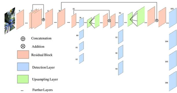
Figure 2. Architecture of YOLO v3
