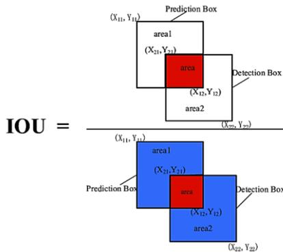
**Figure 7.** Intersection over Union (IoU) calculation diagram.
