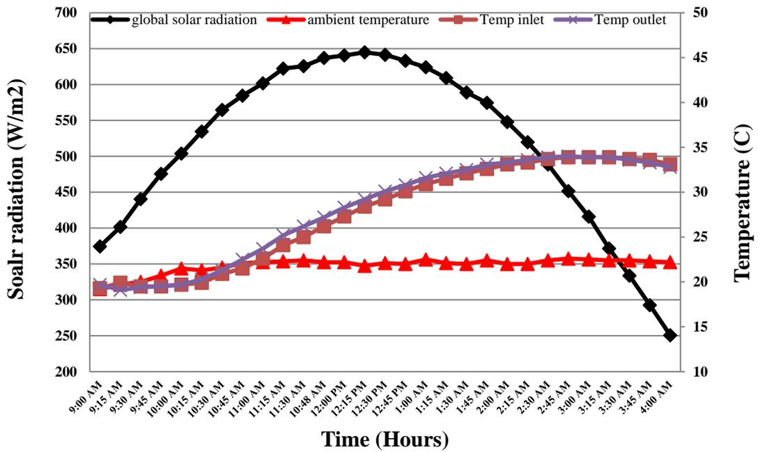
Figure 4. Comparison of ambient temperature,  $T_{inlet}$ , and  $T_{outlet}$  with respect to solar radiation,
