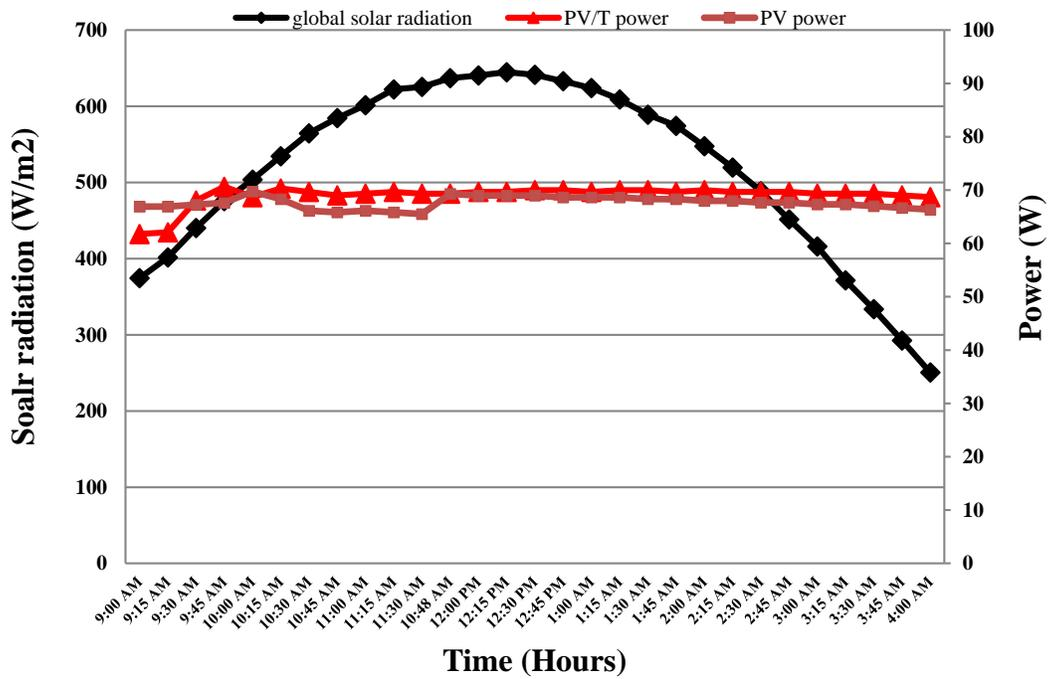
Figure 7. Solar radiation, temperature and PV/T power.
