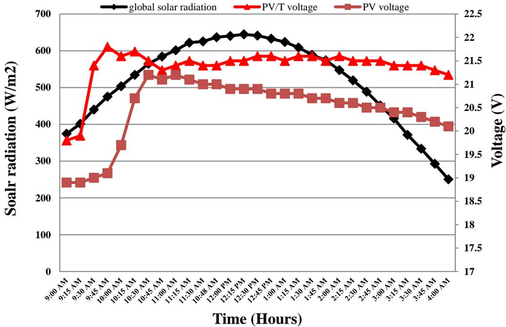
Figure 5. Solar radiation, temperature and PV/T voltage.
