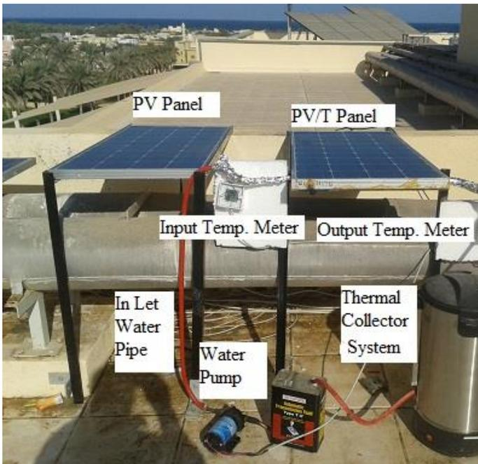
Figure 3. PV/T experimental setup.
