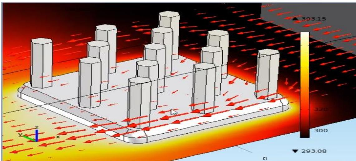
Fig. 7: Air flow through pin fin heat sink
