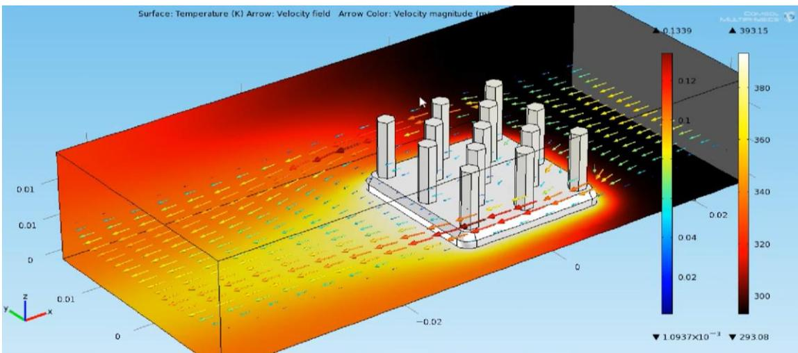
Fig. 6: CFD analysis of pin fin heat sink
