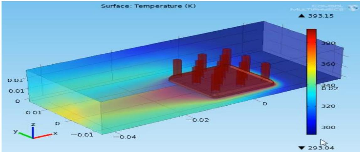
Fig. 5: Temperature distribution inside the channel view
