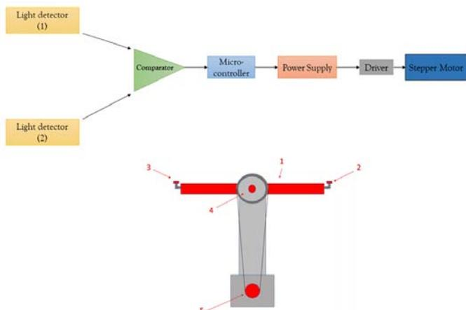
Figure 3: single axis power tracker design (1 PV panel, 2 light detector, 3 light detector, 4 motor pulley, 5 stepper motor).
