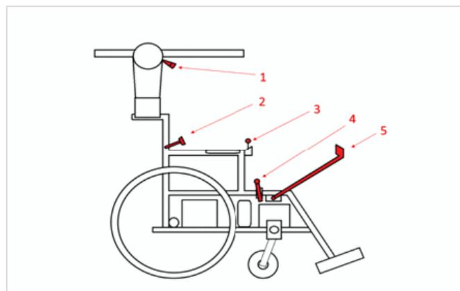
Figure 6: Wheel chair accessories (1 Led light, 2 Fan, 3 Drive control, 4 electric/manual switch, 5 monitor/phone movable-holder)
