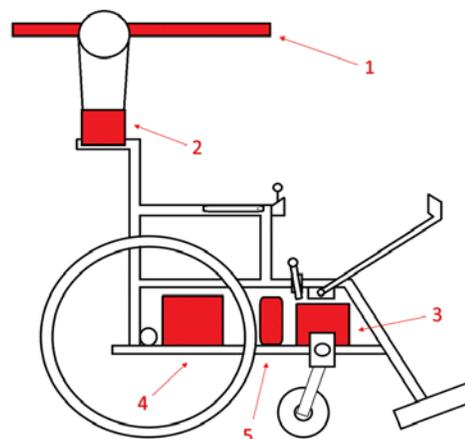
Figure 2: Chair structure for solar power incorporation (1 solar cell, 2 stepper motor, 3 battery, 4 charge controller -with motor case- and 5 Inverter)
