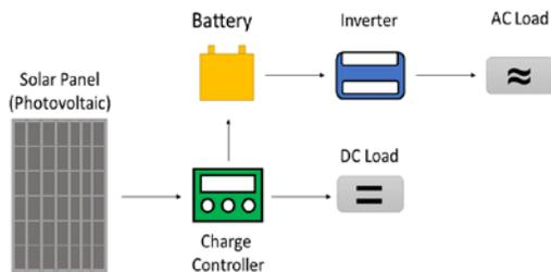
Figure 1. Typical standalone PV system
