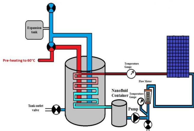
Fig. 1: Schematic diagram of proposed SiC-nanofluid based PVT
