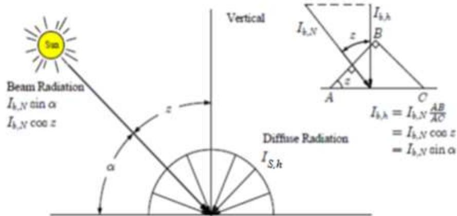
Fig. 1: The solar radiation on a horizontal surface, adapted from [26].
