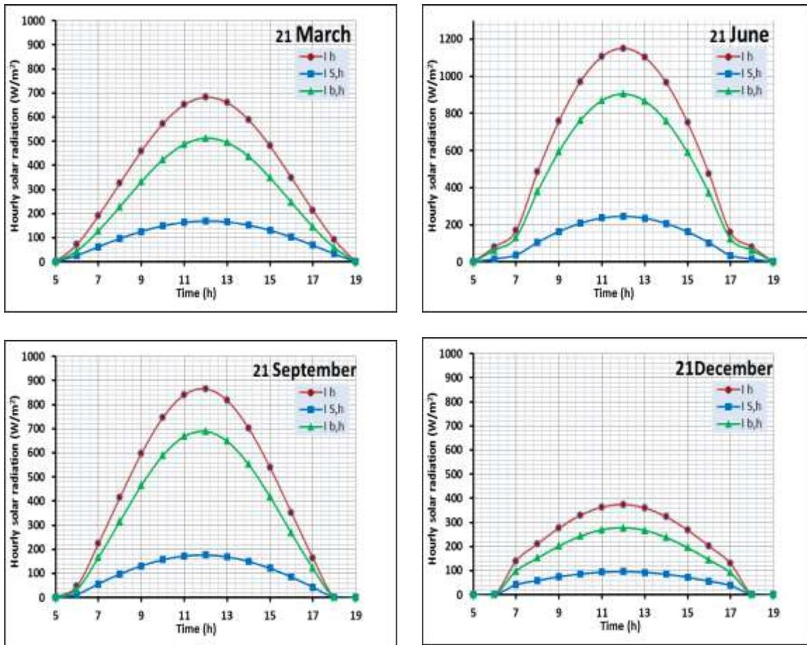
Fig. 3: Changes in the hourly total direct and diffuse solar radiation on a horizontal surface in Baghdad during the 21 March, 21 June, 21September and 21December.
