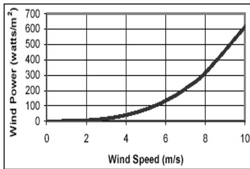
Fig. 3: Relationship between wind speed and wind power
