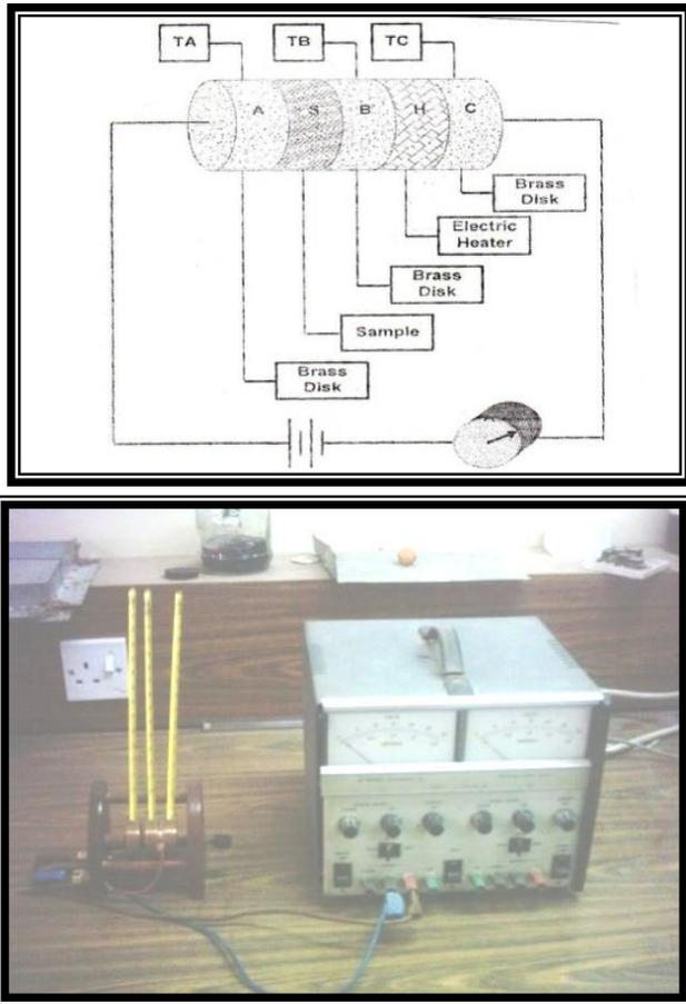
Figure (1): Lee's disc instrument [18]
