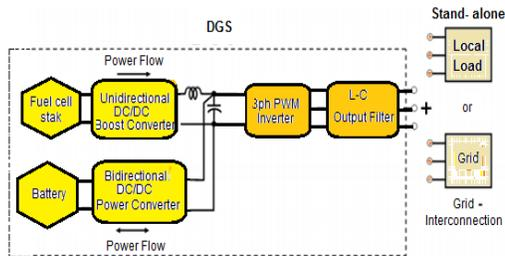
Figure 1 The Two Directional DC/DC Converter (double arrow)
