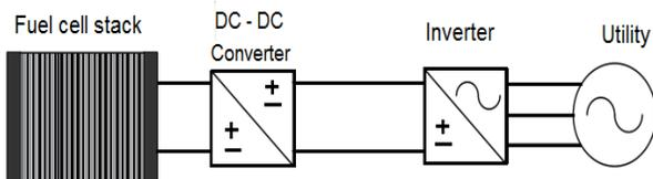
Figure (4): Cascaded Fuel Cell DC-DC and DC-AC Inverter
