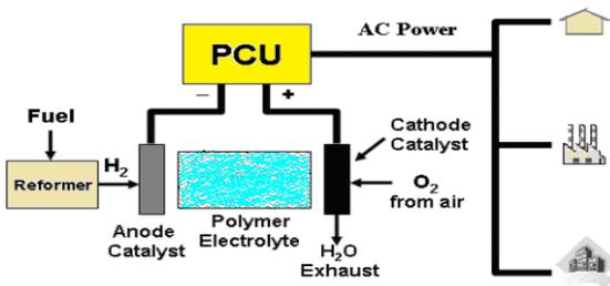
Figure (3): Configuration of the Fuel Cell System
