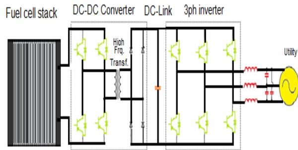
Figure (5): Cascaded DC-DC/DC-AC Converter Topology
