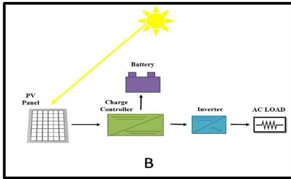
Fig. 2: Block diagram of a simple Stand-alone PV system
