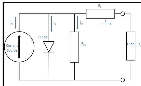
Fig. 1: Electrical circuit representing the PV cell
