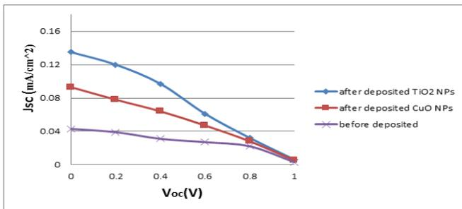
Fig. (13): The photovoltaic performance in dark before deposited and after deposited titanium oxide and copper oxide NPs
