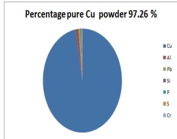
Fig. (4): Percentage pure copper metal powder.
