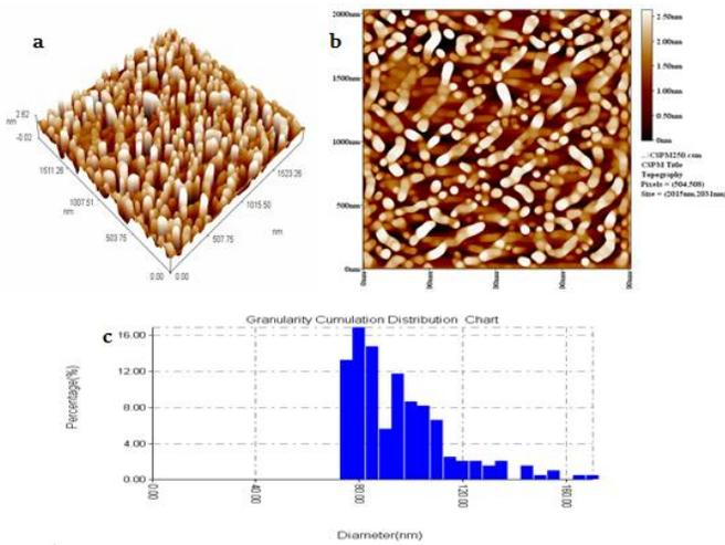
Fig. (6): AFM for titanium oxide.
