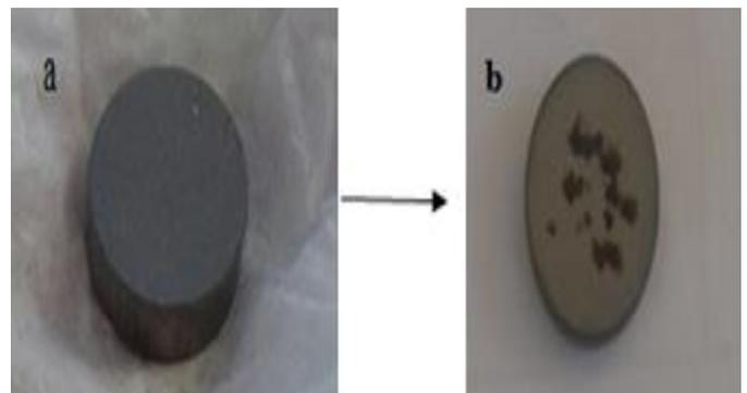
Fig. (5): a)Ti target b) Ti target after laser ablation.
