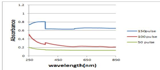
Fig. (12): UV-VIS spectra of copper oxide nanoparticles colloidal in deionized water synthesized at different pulses of laser (50, 100 and 150) respectively.
