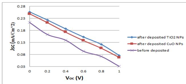
Fig. (14): The photovoltaic performance in illuminated (100mw/cm<sup>2</sup>) before deposited and after deposited Titanium oxide and Copper oxide NPs.
