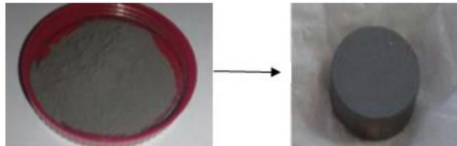
Fig. (1): a) Titanium metal powder b) Titanium powder after pressed with 20 Tons by using hydraulic press.
