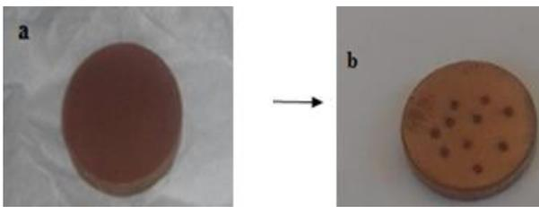
Fig. (8): a) Cu target b) Cu target after laser ablation.
