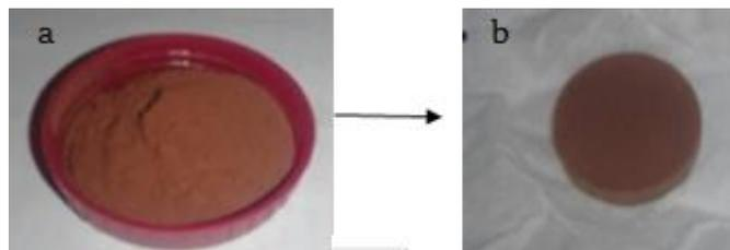
Fig. (2): a) Copper metal powder b) Copper powder after pressed with 20 Tons by using hydraulic press.
