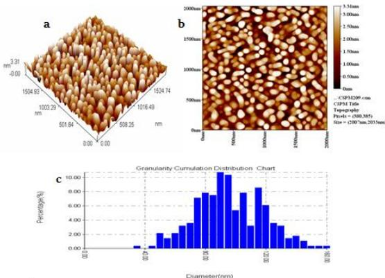
Fig. (9): AFM for copper oxide
