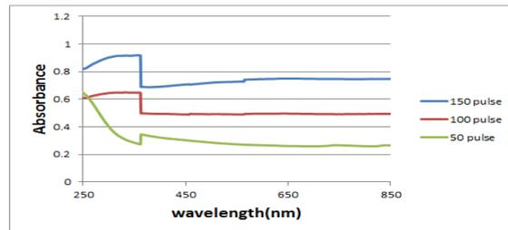
Fig. (11): UV-VIS spectra of titanium oxide nanoparticles colloidal in deionized water synthesized at different pulses of laser (50, 100 and 150) respectively
